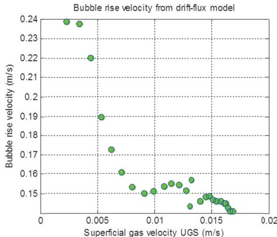
Figure 9. Average bubble rise velocity for PAC 400, based on drift-flux model (Eq.5).
