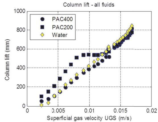
Figure 10. Column lift for all the fluids, static bubbling - without circulation.
