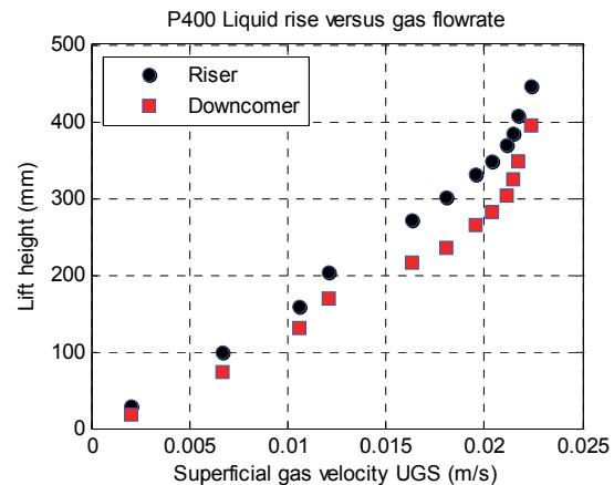
Figure 12. Difference in liquid height in riser and downcomer as a function of gas flow rate. Circulation experiments with fully opened valves using water (top), PAC200 (middle) and PAC400 (bottom).
