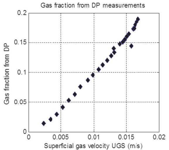
Figure 6. Gas fraction with PAC 400 as a function of superficial gas velocity, based on pressure gradient in riser.
