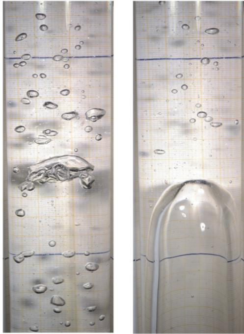
Figure 4. Flow regime in water-filled riser at moderate gas influx varies between bubbly and slug flow. The two images are taken with 2 seconds interval.
