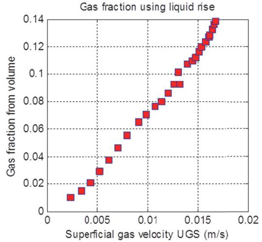
Figure 5. Gas fraction with PAC 400 as a function of superficial gas velocity, based on volumetric increase of liquid in riser is used.
