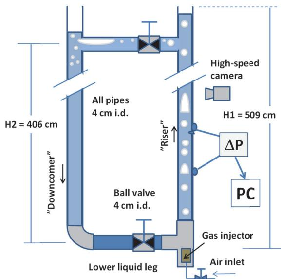
Figure 1. Sketch of the gas-lift loop, with definitions of “Riser”, “Downcomer” and crossover “Legs”.
