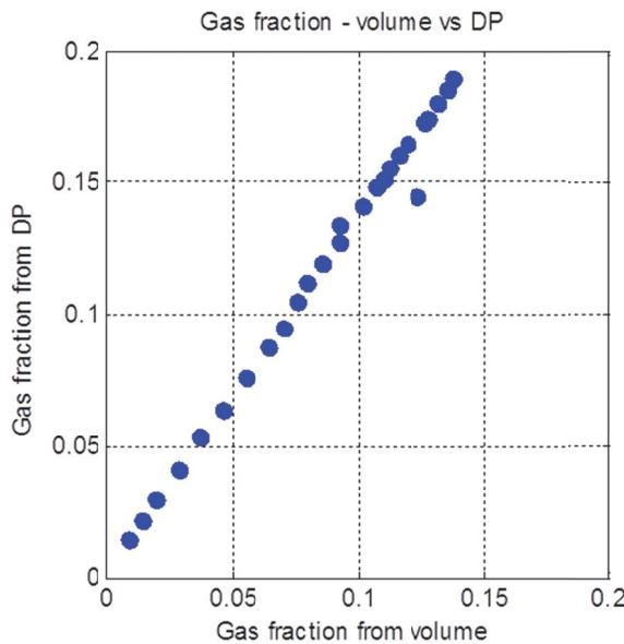
Figure 7. Gas fraction with PAC 400 – volumetric method versus pressure.
