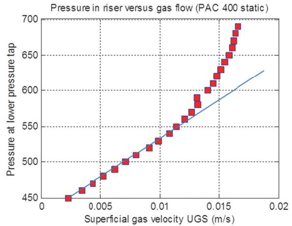
Figure 8. Gauge pressure (in mbar) at bottom of riser as a function of gas inflow rate for PAC 400.
