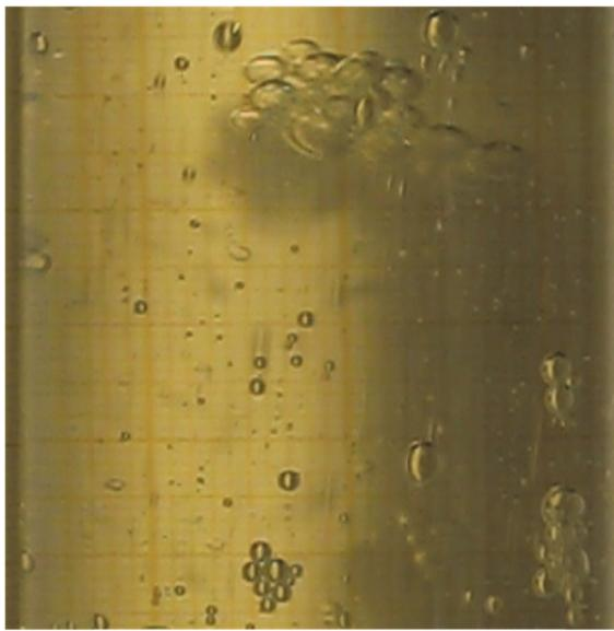
Figure 11. Flooding of gas bubbles into the downcomer with PAC 400 liquid. The bubbles agglomerate, rotate and rearrange in constantly varying patterns. Image snapshot from video.
