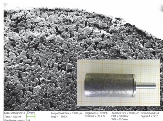
Figure 2. Picture of the gas injector inserted into an electron microscope image of the surface. Magnification is 100X, and the image width is approximately 3.8 mm.
