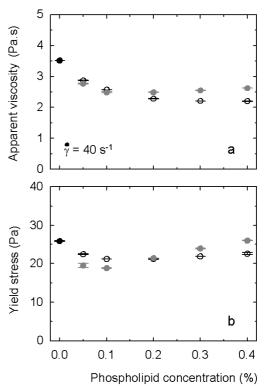
Fig 2. Apparent viscosity (a) and yield stress
