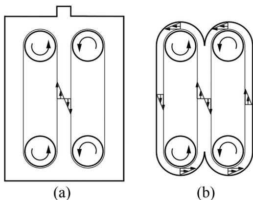
Figure 1. a) Taylor's parallel band instruments, b) The present design.
