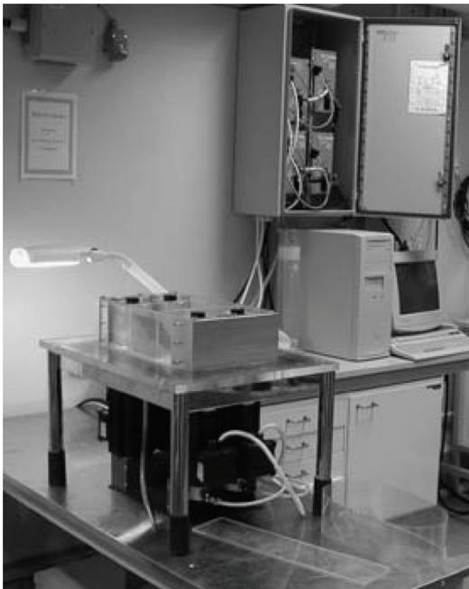
Figure 5. The parallel band instrument, with electronics and computer system in the background.
