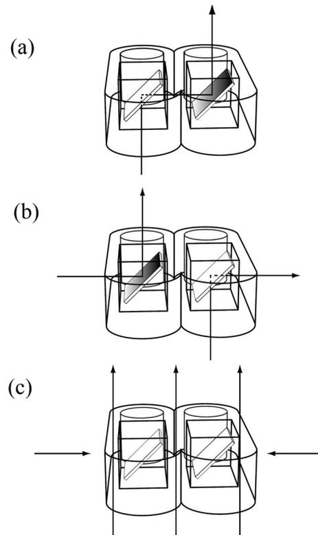
Figure 3. Observation and illumination directions. a) In shear direction central region. b) In the shear direction, outer region, and c) In the indifferent direction.
