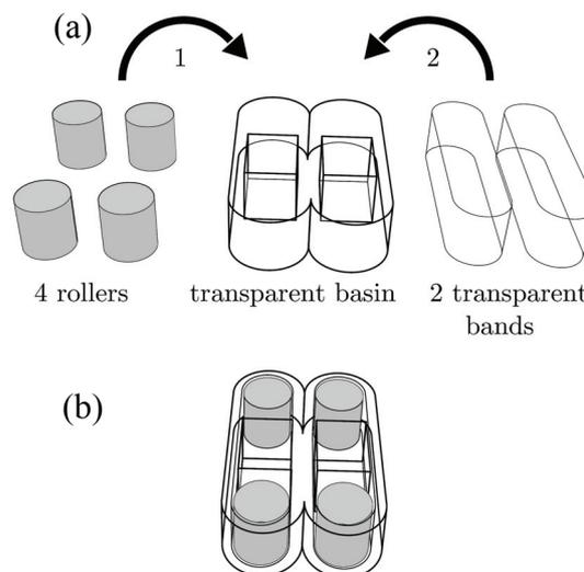
Figure 2. The band rheometer, principally. a) The main components consist of a transparent basin with two observation shafts, four rollers and two transparent bands, b) The assembled band instrument.
