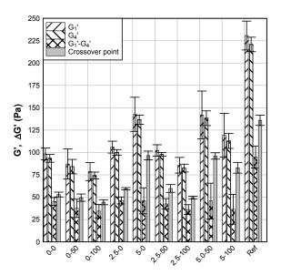
Figure 2. G<sub>1</sub>', G<sub>4</sub>', G<sub>1</sub>'-G<sub>4</sub>' and G'<sub>Crossover</sub> for the different recipes. The error bars indicate plus/minus 1 standard deviation.
