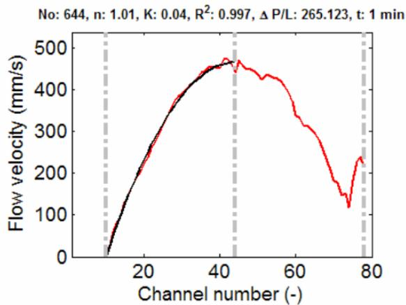
Figure 3. Instantaneous velocity profile (red solid line) with corresponding power-law fit (black solid line) for stationary flow of sunflower oil.
