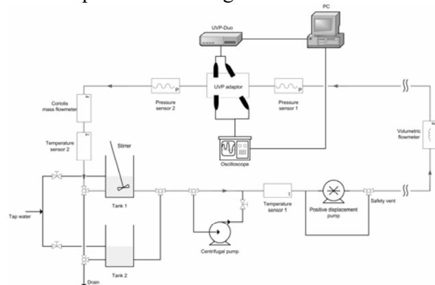
Figure 1. Schematic illustration of the experimental flow loop and instrumentation.
