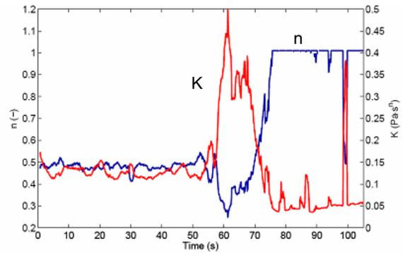
Figure 4. Corresponding variation in power-law parameters  $n$ ,  $K$ , for the transition from Xanthan to sunflower oil.
