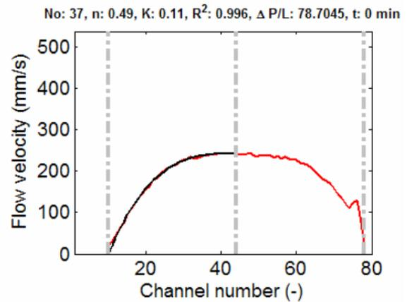
Figure 2. Instantaneous velocity profile (red solid line) with corresponding power-law fit (black solid line) for stationary flow of Xanthan.
