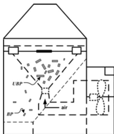
Figure 2. Borregaard pellet durability tester. The figure has been modified from Payme, J.D.<sup>5</sup> to indicate where the unbroken pellets (*UBP*) and broken pellets (*BP*) are situated.
