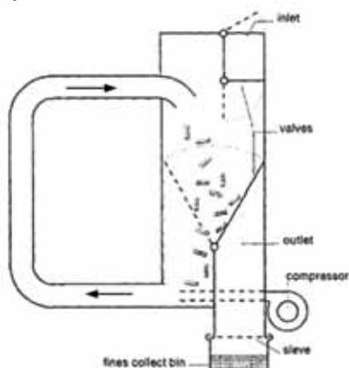
Figure 1. Holmen durability pellet tester.<sup>2</sup>
