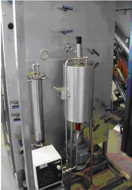
**Figure 1: The Dispersion Characterization Rig with the Dispersion Characterization Probe (DCP) in the centre.**
