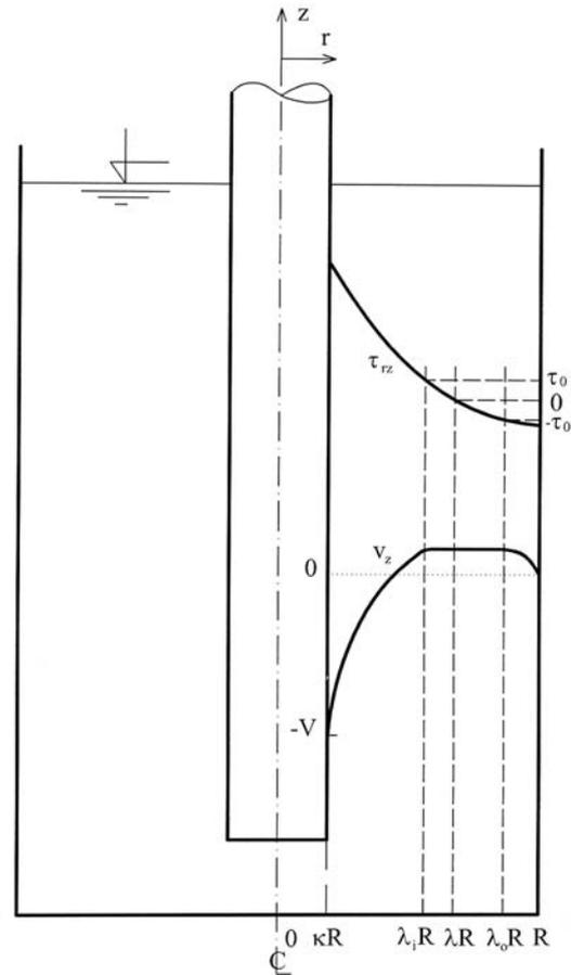
Figure 1. Definition sketch of a back extrusion.
