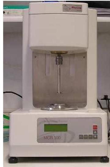
Figure 1: Rheometer MCR 300
