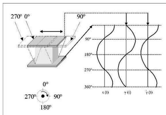
Figure 3. Principle of oscillatory tests within the LVE deformation range according to Maxwell (Mezger 2002).
