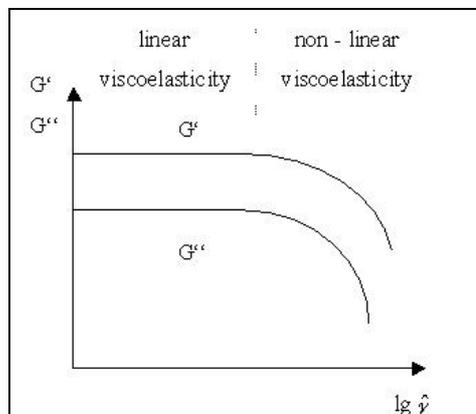
Figure 4. Graphs of  $G'$  and  $G''$  represent the relation of stored to lost elastic behaviour, depending on the shear rate, here, or on the angular frequency, where the linear viscoelastic (LVE) deformation range is defined (dotted line) (according to Mezger 2002).
