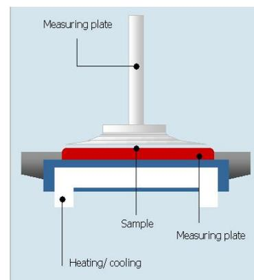
Figure 2: PP MS with Peltier unit
