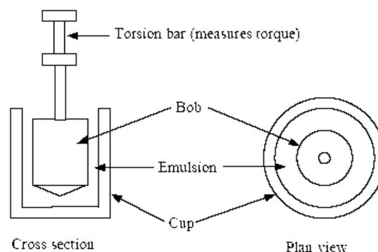
**Figure 1: Measuring principle of bob/cup measuring system.**
