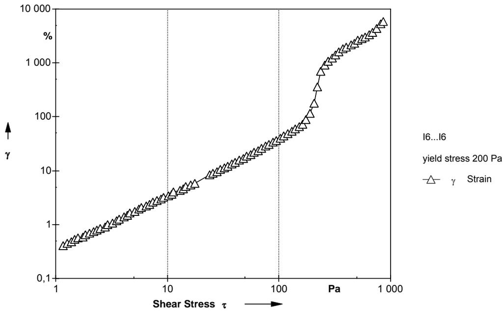
Figure 7: Diagram of strain versus shear stress showing yield at 200 Pa, CC26.61Pr/Ti.
