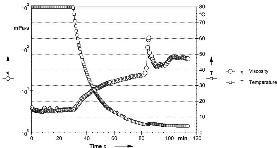
Figure 3: Temperature and viscosity during hydrate formation in a constant pressure test, CC26.61Pr/Ti.
