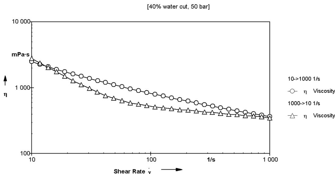
Figure 5: Viscosity versus shear rate at 1 °C. Viscosity is 2500 mPas at 10 s<sup>-1</sup> and 364 mPas at 1000 s<sup>-1</sup> (increasing shear rate shown by circles). Viscosity is 350 mPas at 1000 s<sup>-1</sup> and 2788 mPas at 10 s<sup>-1</sup> (decreasing shear rate shown by triangles), CC26.61Pr/Ti.
