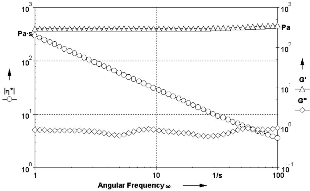
Figure 6: Complex viscosity,  $G'$  and  $G''$  versus frequency for solidified sample, CC26.61Pr/Ti.
