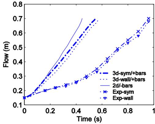
Figure 6. Simulation and experiments of Bingham fluid in the L-box.  $\tau_0 = 39$  Pa,  $\eta_{pl} = 5$  Pa·s. Sym = plane of symmetry. Wall = flow at the boundary,  $z = 0$  and  $z = -200$  mm. /-bars = no reinforcement. /+bars = reinforcement. Exp = experiment.
