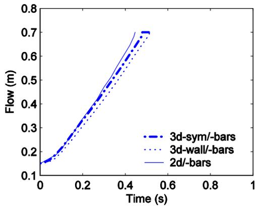
Figure 7. Simulation of the L-box for a Bingham fluid.  $\tau_0=39$  Pa,  $\eta_{pl}=5$  Pa·s. Sym = plane of symmetry. Wall = flow at the boundary,  $z = 0$  and  $z = -200$  mm. /-bars = no reinforcement.
