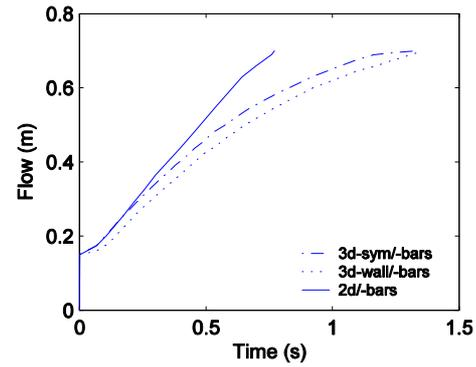
Figure 4. 2-d and 3-d simulation of flow into horizontal section of L-box (no reinforcement).  $\eta = 20$  Pa·s. Sym = plane of symmetry. Wall = flow at the boundary,  $z = 0$  and  $z = -200$  mm. /-bars = no reinforcement. /+bars = reinforcement.
