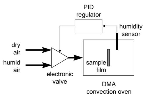
Figure 1. Sketch of the humidity control system.
