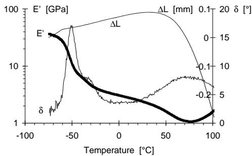
Figure 2. Storage modulus  $E'$ , phase angle  $\delta$ , and length increase  $\Delta L$  of a grease-covered plasticized amylose film.
