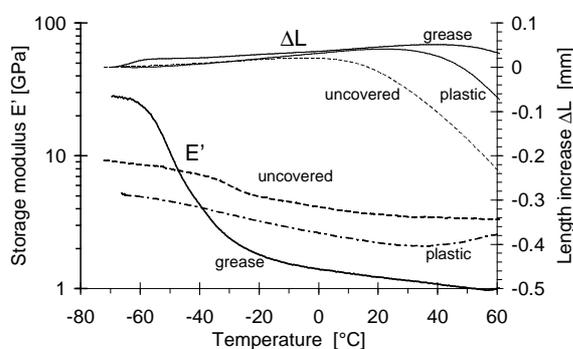
Figure 3. Storage modulus  $E'$  and length increase  $\Delta L$  of plasticized amylose films covered with grease, covered with plastic film and uncovered.
