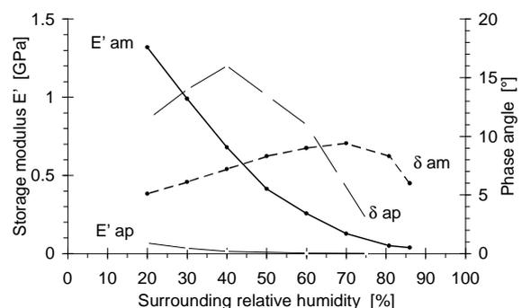
Figure 4. Storage modulus  $E'$  and phase angle  $\delta$  of a plasticized amylose (am) and amylopectin (ap) films at 25 °C.
