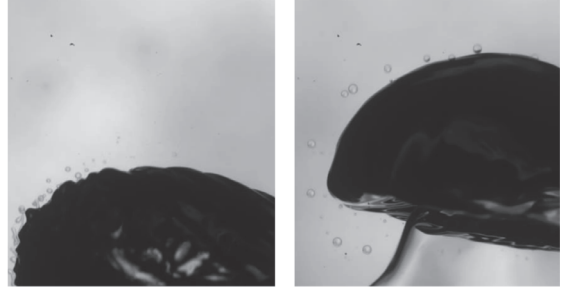
Figure 7: Selected snapshots from the high speed images of the bubble shape at the interface. Left: liquid drainage on top of the bubble. Right: the bubble drifts in a thin filament
