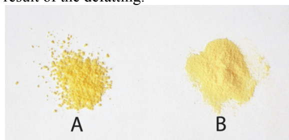
Figure 1. The pure zein as powder. A shows the zein before defatting, B shows the defatted zein.
