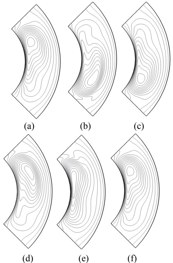
Figure 7. Isotherms in a period for  $Re=1$ ,  $We=1$ ,  $\omega_r=0.55$ ,  $Pe=900$ ,  $Br=50$ ,  $\varpi=0.3$ ,  $\varepsilon=1$  and  $A=5$ .
