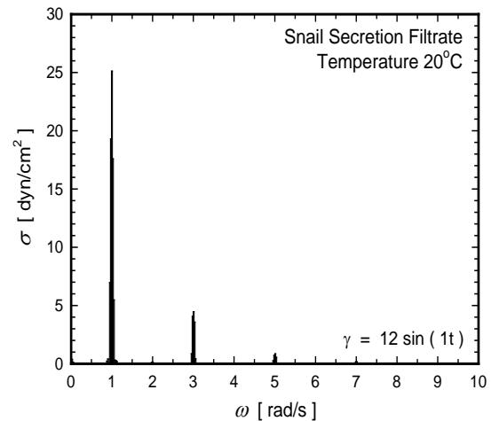
Figure 4. Fourier spectrum of nonsinusoidal response for snail secretion filtrate.
