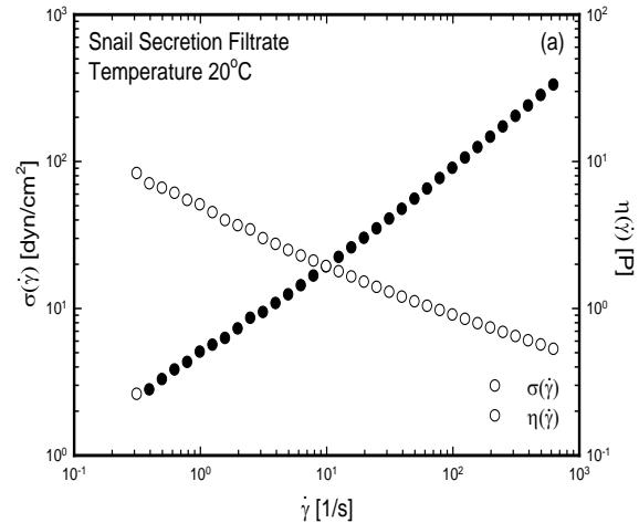
Figure 1. Shear stress and steady shear viscosity versus shear rate for snail secretion filtrate.
