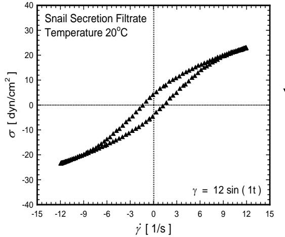
Figure 3. Lissajous curve for snail secretion filtrate at strain amplitude amplitude of 1200 %.
