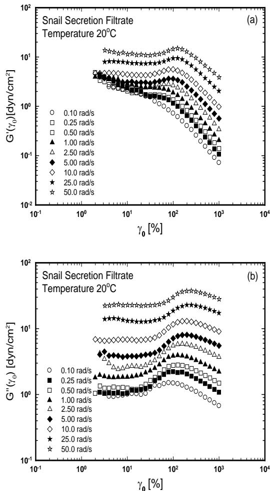
Figure 2. (a) Storage modulus and (b) loss modulus as a function of strain amplitude for snail secretion filtrate with different angular frequencies.
