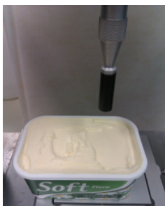
Figure 3. The Texture Profile Analyser TA-HDi TPA showing the PO 5R ½" Delrin BS 757 probe.
