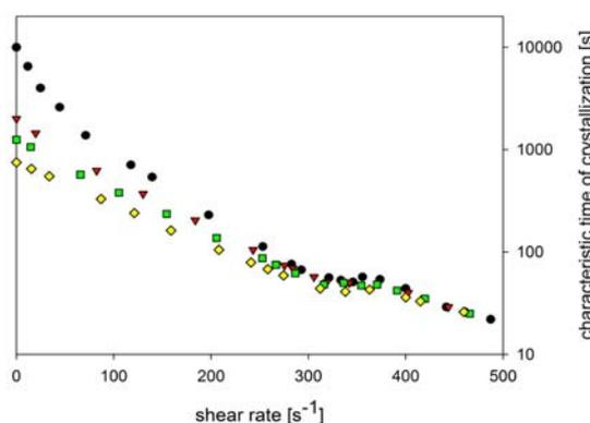
figure 3: Characteristic times as a function of shear rate (circles: neat polymer, triangles particles with aspect ratio 1, squares aspect ratio 1.8 and diamonds aspect ratio 3.6).
