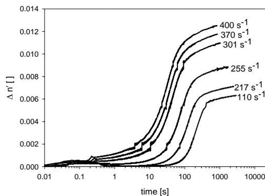
Figure 2: evolution of the birefringence after cessation of flow (different shear rates, strain=100,  $145^\circ\text{C}$ )
