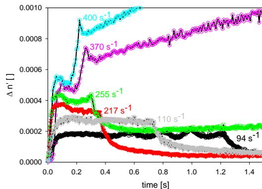
Figure 1: Birefringence evolution during the application of flow (different shear rates, strain=100,  $145^\circ\text{C}$ )
