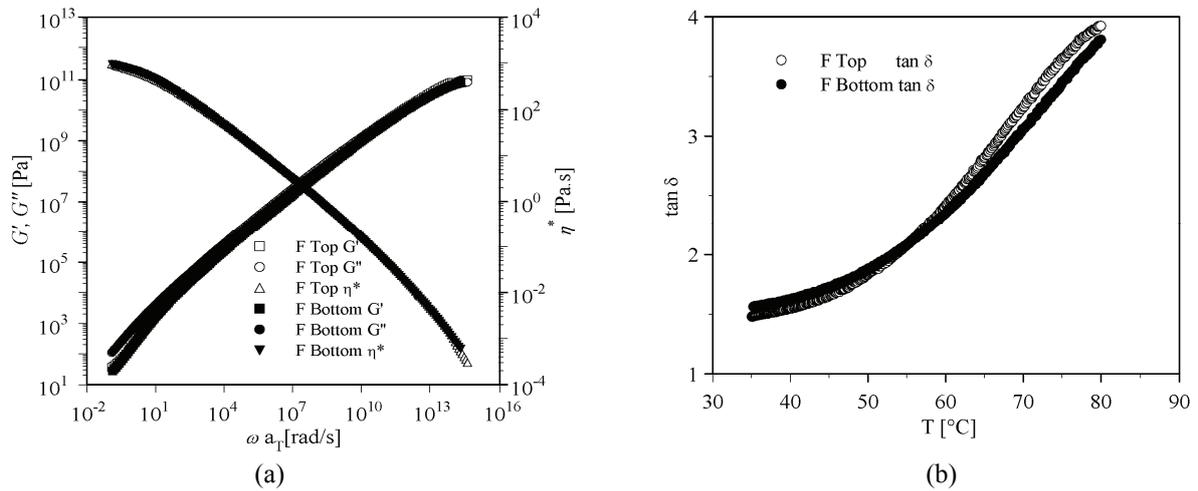
Figure 2. (a) Storage and loss moduli and complex viscosity of sample F. containing 2.5% SBS and 10% crumb-rubber (reference temperature 60°C) and (b) Loss tangent,  $\tan \delta$  of bottom and top parts obtained by a temperature sweep.
