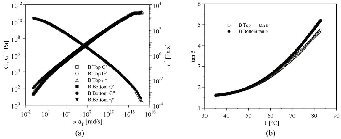
Figure 1. (a) Storage and loss moduli and complex viscosity of sample B containing 0.7% SBS and 10% crumb-rubber (reference temperature 60°C) and (b) Loss tangent  $\tan \delta$  of bottom and top parts obtained by temperature sweep tests.
