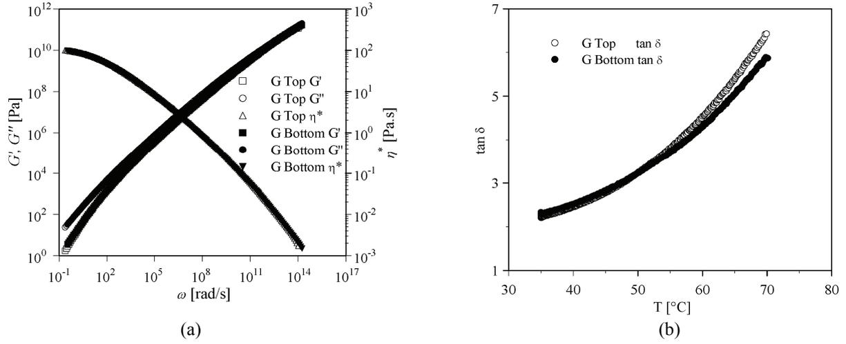
Figure 3. (a) Storage and loss moduli and complex viscosity of sample G. with 0.7% SBS and 10% crumb-rubber (reference temperature 60°C) and (b) Loss tangent,  $\tan \delta$  of bottom and top parts obtained by a temperature sweep
