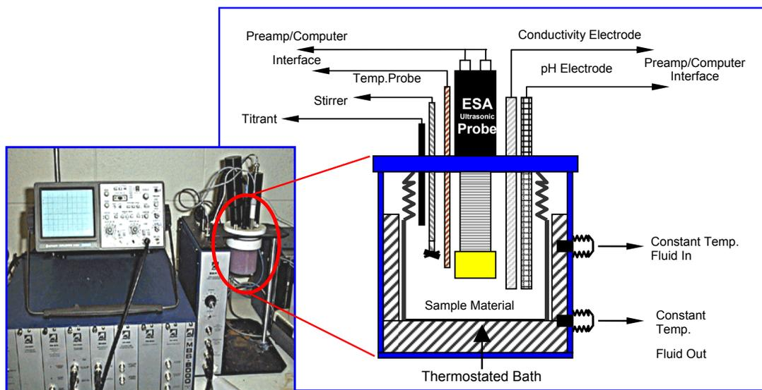
Figure 1. ESA-8000 system (Matec, Applied Science, USA) included by its SSP-1 sample Cell, as a new tool for zeta potential measurements of carbon fibers.
