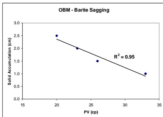
Figure 4. Solid accumulation vs. plastic viscosity of OBM sample.
