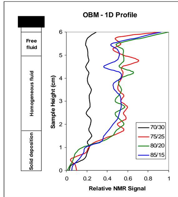
Figure 3. 1D profile of OBM sample.
