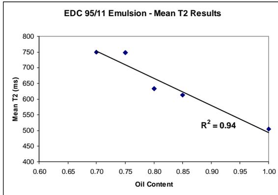
Figure 1. Mean T2 results of EDC 95/11 and water emulsions.
