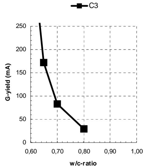
Figure 3. Effect of w/c-ratio on rheology
