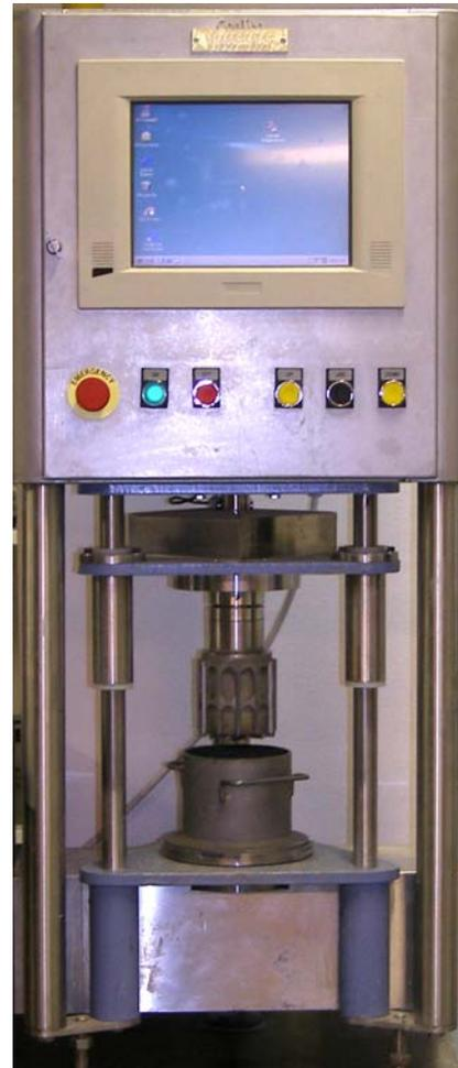
Figure 1. ConTec Viscometer 6
