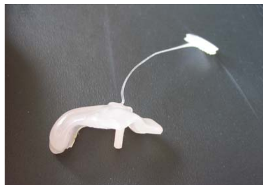
Figure 6. Molten sample still showing the good grip of the clamps
