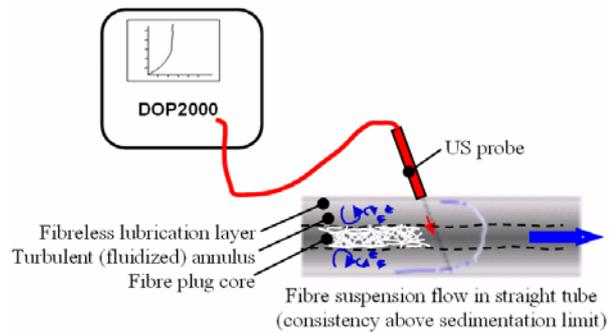
Figure 2. The pulsed ultrasound Doppler velocimeter (Signal Processing-DOP2000).
