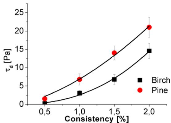
Figure 7. The disruptive shear stress  $\tau_d$  as a function of consistency for pine and birch fiber suspensions. The solid lines give the fitted values according to Eq. 3.
