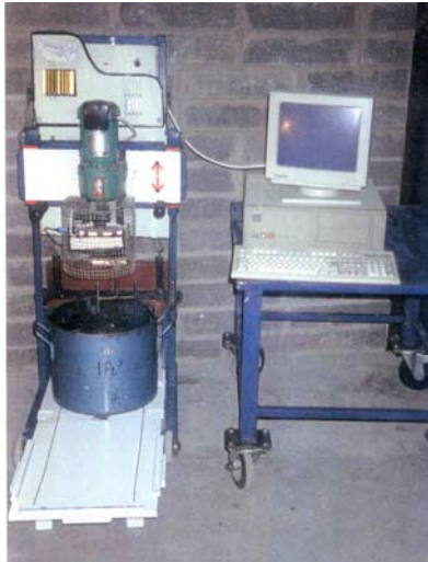
Figure 3. The TCD two point workability apparatus 14 .
