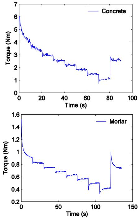
Figure 2. Rheological measurements on concrete and mortar.
