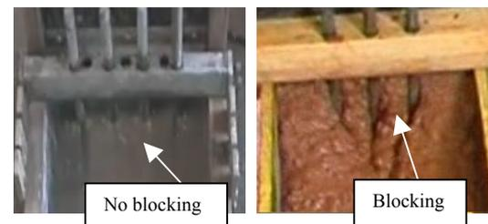
Figure 5. Flow of mortar (left) and concrete (right) near the reinforcement in the L-box.
