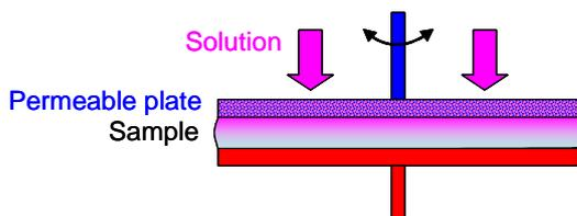
Figure 2. The principle of permeable plate rheometry.
