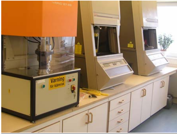
Fig. 8 Instruments to measure cure behaviour; Gottfert, Monsanto MDR and Monsanto ODR
