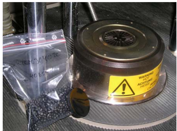
Fig. 6 Monsanto Moving Die Rheometer, MDR, die with pellets and compression moulded specimen.
