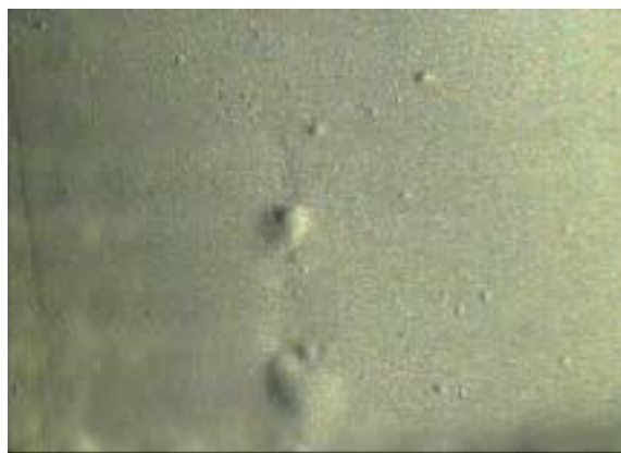
Figure 3. Hot oil test, example of lump in inner semiconductive layer, width 0.5 mm, height 0.05-0.1 mm.
