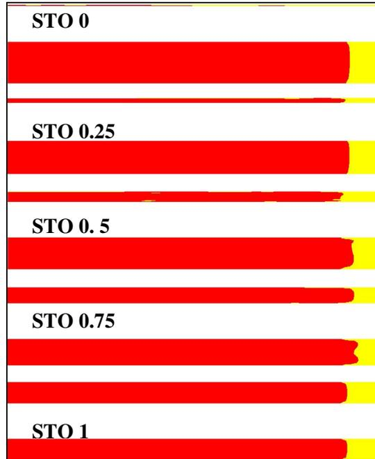
**Figure 7:** Cement (red) displacing Spacer (yellow). Minimum flow rate,  $Re= 4.04$ .
