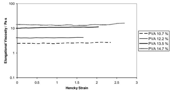
Figure 5a,b and c. Filament stretching results on solutions of CMC (top), ASE (centre) and PVA (bottom). Extensional viscosity is also here given as a function of the Hencky strain.
