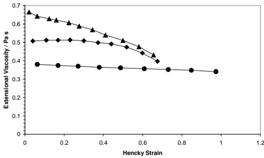
Figure 4. Results from filament stretching measurements of the coating colours containing CMC (◆), ASE (▲) and PVA (●). Extensional viscosity is given as a function of Hencky strain.
