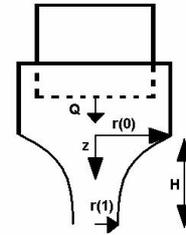
Figure 1. Side view of the converging channel-flow measuring cell
