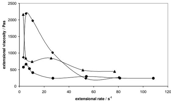
Figure 3. Results from the converging channel-flow measurements of the coating colours containing CMC (◆), ASE (▲) and PVA (●), respectively
