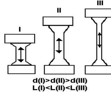
Figure 2. Idealised view of stretching of a fluid filament at times I to III. The length ( $l$ ) is constant at times after III, whereas the diameter ( $d$ ) continues to decrease until rupture of the filament.
