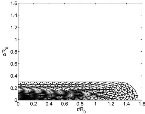
Figure 1: Mesh which has been deformed 70%. Original geometry was the cross-section of a quarter sphere.
