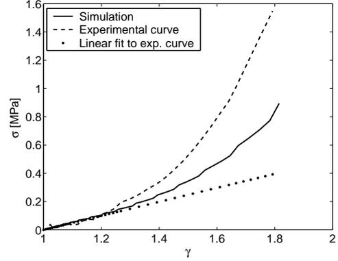
Figure 2: Comparison of a simulated curve with an experimental curve. Also shown is the a linear fit to the experimental curve up to  $\gamma = 1.10$ . Simulation was carried out with  $\mu = 1.2 \cdot 10^4 Pa \cdot s$  and  $G = 1.2 \cdot 10^5 Pa$ .
