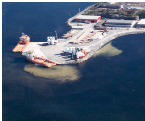
Figure 1. Accidental discharges while loading barite at Florø base. (Photo: Are Fjellstad, Florø 1989)
