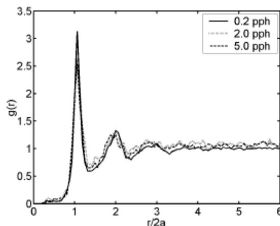
Figure 7. The  $g(r)$ -curves for the dry EHEC-containing PS layers at 55°C. The radial distance is normalized with respect to the particle diameter ( $2a$ ).
