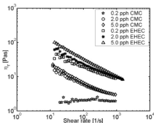
Figure 3. The relative viscosity of the CMC/EHEC-containing suspensions vs. shear rate. Temperature 23°C.
