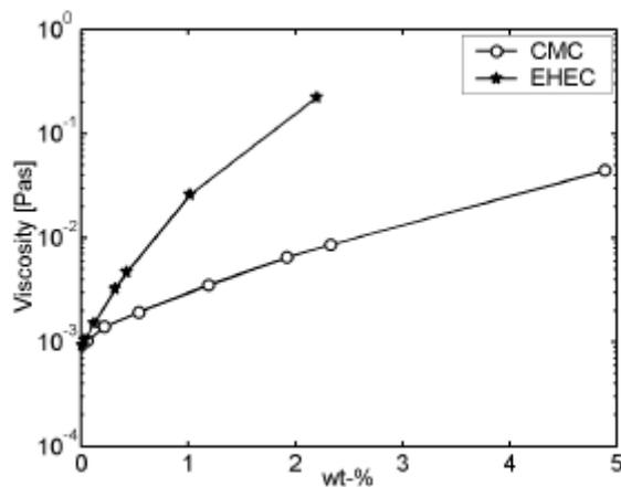
Figure 1. The viscosity vs. the concentration of cellulose ether. Aqueous solutions at 23°C and pH=8.
