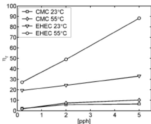
Figure 5. The relative viscosity of the PS suspensions vs. the amount of water-soluble polymer added, at a shear rate of  $100 \text{ s}^{-1}$ .
