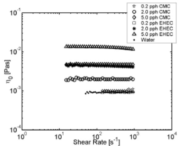
Figure 2. Aqueous phase viscosities of the PS-suspensions. Pure water is included as a reference. Temperature 23°C.
