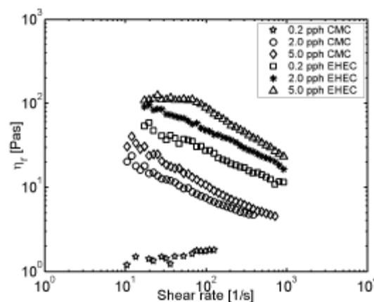
Figure 4. The relative viscosity of the CMC/EHEC-containing suspensions vs. shear rate. Temperature 55°C.
