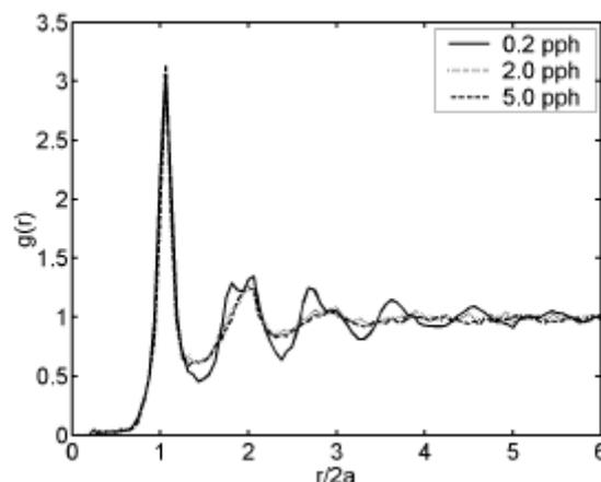
Figure 6. The  $g(r)$ -curves for the dry CMC-containing PS layers at 55°C. The radial distance is normalized with respect to the particle diameter ( $2a$ ).
