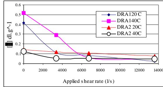
Figure 4  $[\eta]$  for the different sets of the applied shear rates on DRA1 and DRA2 at 20 and 40°C.
