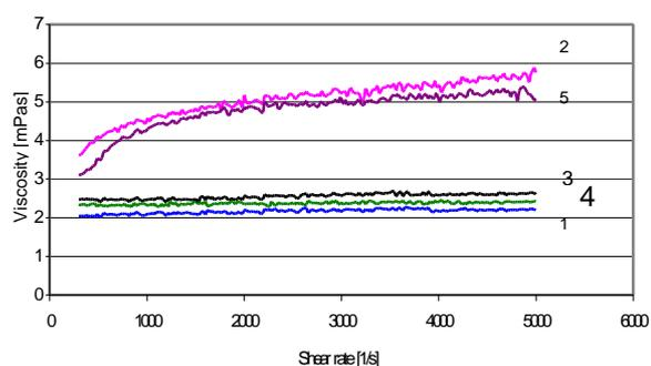
Figure 2 Viscosity of 1000 ppmw DRA1 exposed to different shear rates at 40C,
