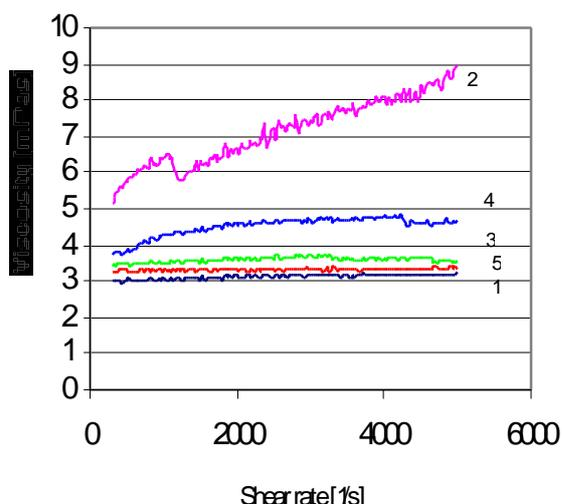
Fig.1 Viscosity of 1000 ppmw DRA1 exposed to different shear rates at 20C
