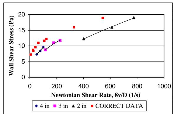
Figure 5 – Slip Correction – 300 psig / 100F / 80% Quality – Baseline Tests
