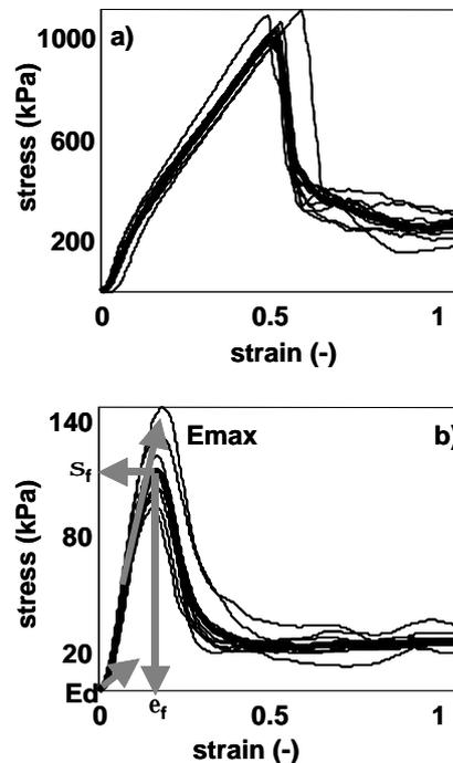
Fig. 2. Stress-strain compression curves for one potato sample in ten replicates in a) raw and b) cooked state.
