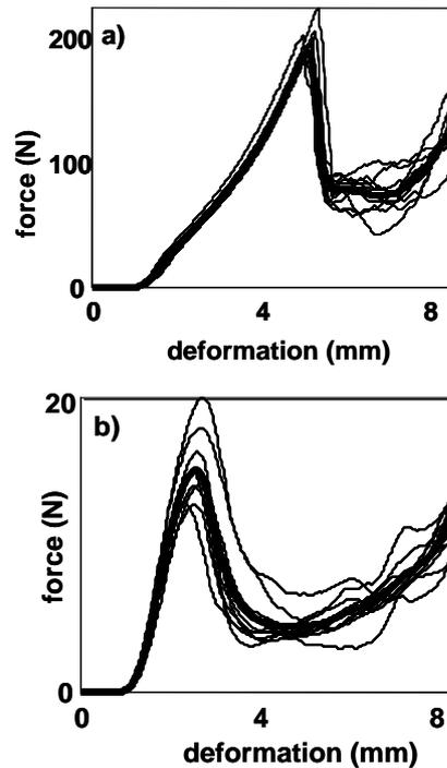
Fig. 1. Force-deformation compression curves for one potato sample in ten replicates in a) raw and b) cooked state. (thin line: ten replicates, bold line: average)
