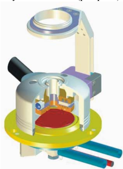
Figure 4b: Drawing of the Advanced Peltier System PTD 150 (pat. pent.)
